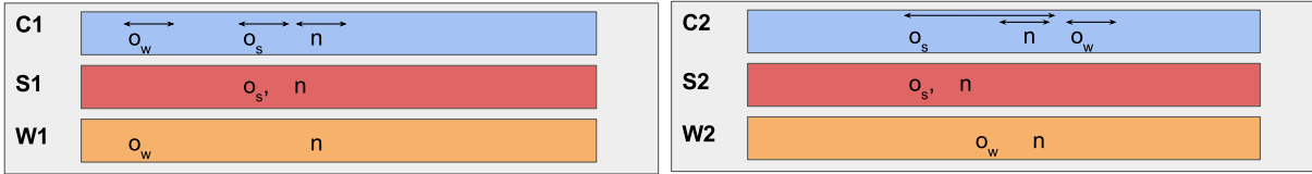
Figure 4: The gray boxes labeled with clients C_1 and C_2 contain three different timelines; the blue timeline corresponds to events as observed by the client, the red timeline indicates when data at S became available to the client, and the orange timeline indicates when data at W became available to the client. In this scenario, we observe that data at S becomes available to both clients simultaneously, while data written to W by C_1 can be delayed before it becomes available at W for C_2 .
