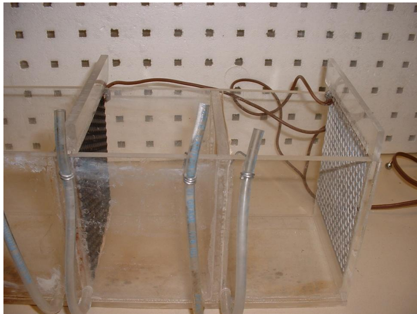
Figure 2.2 Electrochemical pH adjustment apparatus.
