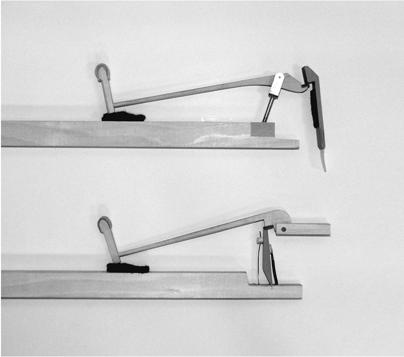
Figure 1 Prellmechanik (top) and Stossmechanik (bottom)
