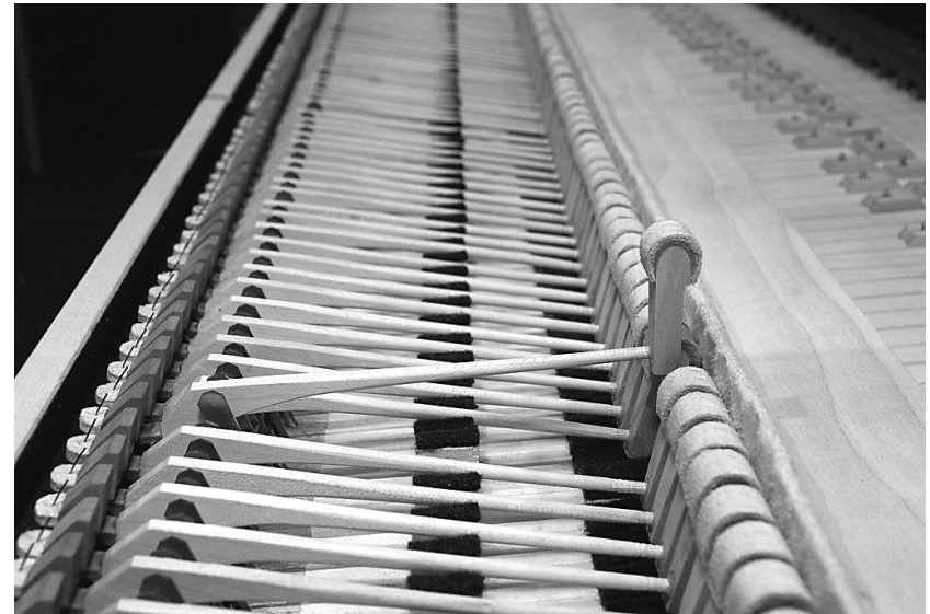
Figure 2 (b) prell-hammer nearing escapement
