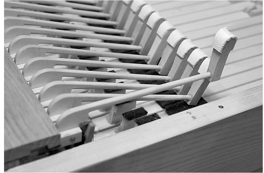
Figure 2 (a) stoss-hammer nearing escapement
