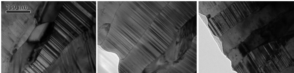
Figure 3.4: TEM images of thin film sample cross-sections showing nanotwins in grains; deposition rates for samples presented are (a) 1.1 nm/s, (b) 3.6 nm/s and (c) 11.2 nm/s
