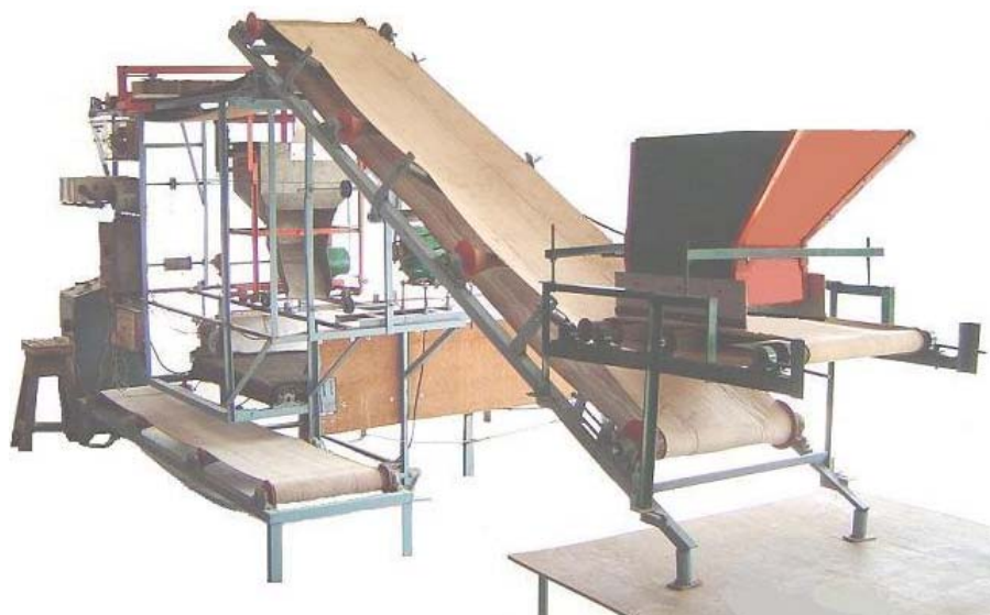
Figure 4. The developed model of mechanical loading-unloading cum withered-leaf shifting system for a withering trough
