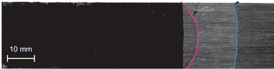
Non-self-similar crack growth in mixed-mode bending specimen
