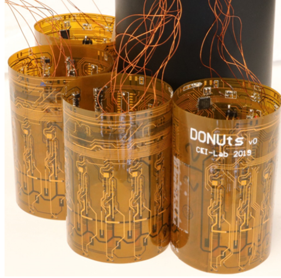
Figure 7.3: Four DONUt modules encapsulating an obstacle. Modules have onboard actuation, sensing, communication, and computation.
