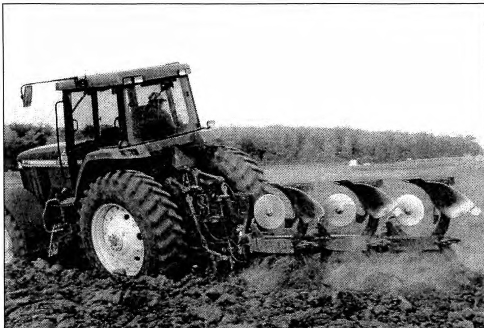
With recent state appropriations, the Field Research Unit was able to upgrade field research equipment, including the replacement of several 1950 vintage tractors, and the purchase of a 'Deep Till' plow (shown here) which allows them to break up compacted soil early in the season when it is still wet.
