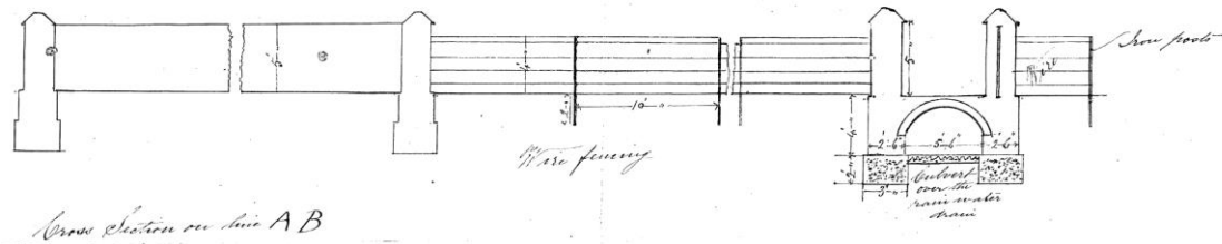
Figure 4.13: Side-view of path to Parsi burial ground with proposed culvert over drain. 427
