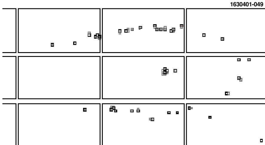
Figure 2.4: Example of hits produced by a Cherenkov cone in the RICH detector. The charged particle also produces a cluster at the center of the cone.
