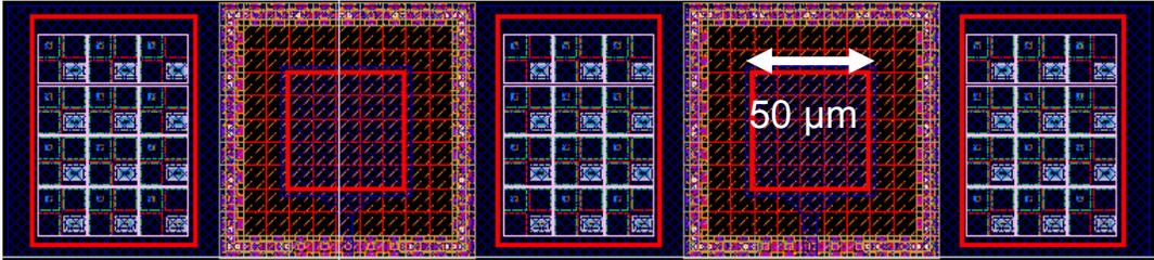
Figure 2.3: 100  $\mu\text{m}$  Pitch GSGSG Pad Array with 50  $\mu\text{m}$  x 50  $\mu\text{m}$  Signal Pad
