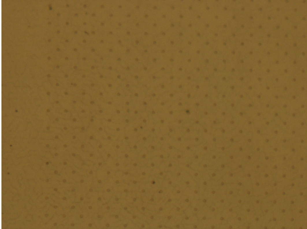
Figure 2.2: Example of the “Ohmic Claw” holes etched into ohmic layer after the device isolation etch step. The holes are 1 \mu\text{m} in diameter.
