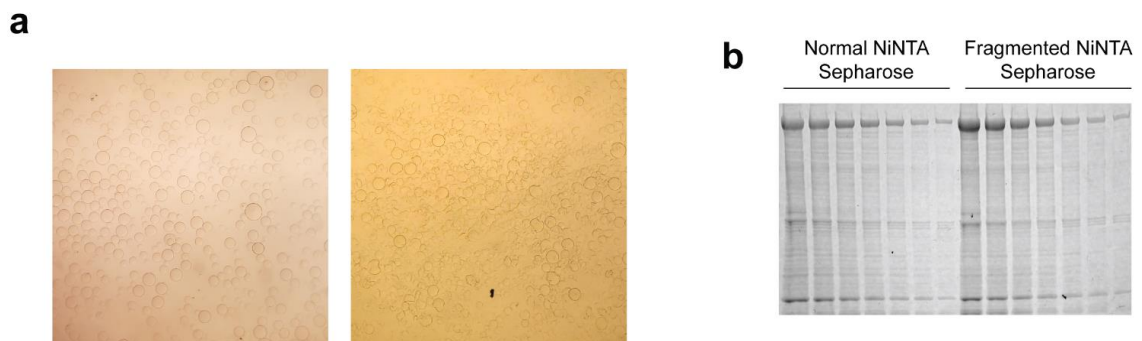
Figure 2.16 – Fragmented NiNTA resin improves purification yield. a , DIC microscopy image (4x magnification) showing thermofisher HisPur resin (Cat. no. 88221) before (left) and after (right) 3 minutes of sonication. b , Parallel purifications using standard or fragmented resin.
