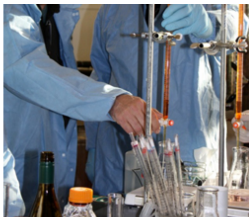
Iodine is used in the titrametric 'Ripper' method for measuring SO 2
