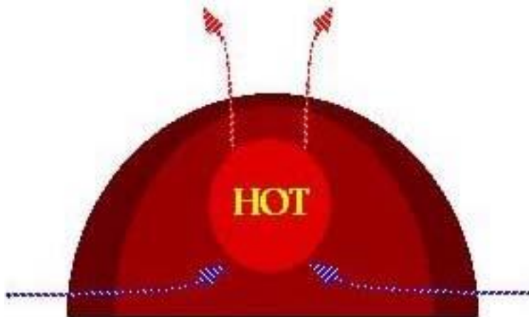
Figure 1. Natural Air Circulation in a Compost Windrow
