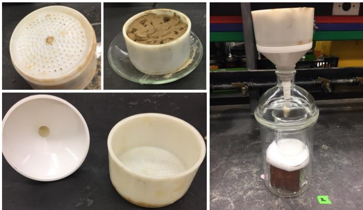
Figure 4.1. Buchner funnels and pump used in the leaching experiment.
