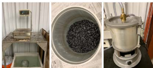
Fig. 7. Theoretical maximum specific gravity test
