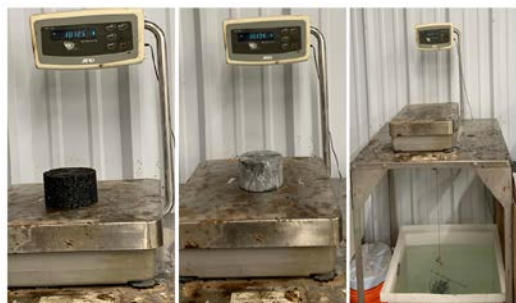
Fig. 8. Paraffin-method based bulk specific gravity test
