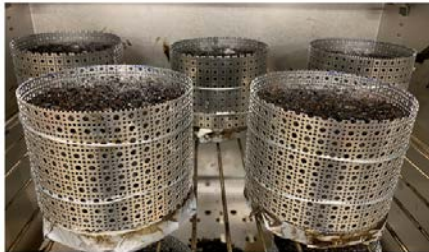
Fig. 21. Curing process of BEAB-based OGFC specimens
