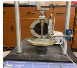
Fig.9. Marshall stability test for OGFC specimens
