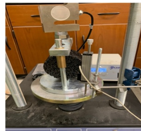
Fig. 10. Indirect tensile test for OGFC specimens
