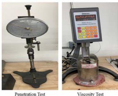
Fig. 6. Penetration and viscosity test for asphalt binder
