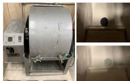
Fig. 11. Cantabro loss test for OGFC specimens
