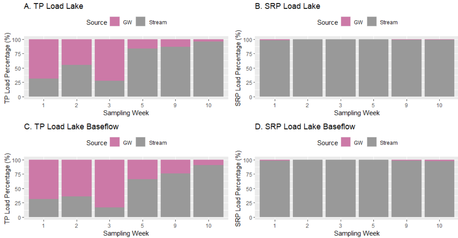
Figure 17. TP (A, C) and SRP (B, D) loading proportions from groundwater (pink) vs streams (grey) on a weekly basis at Oneida Lake during summer 2020. Bottom figures (C, D) represent the load during baseflow conditions only.
