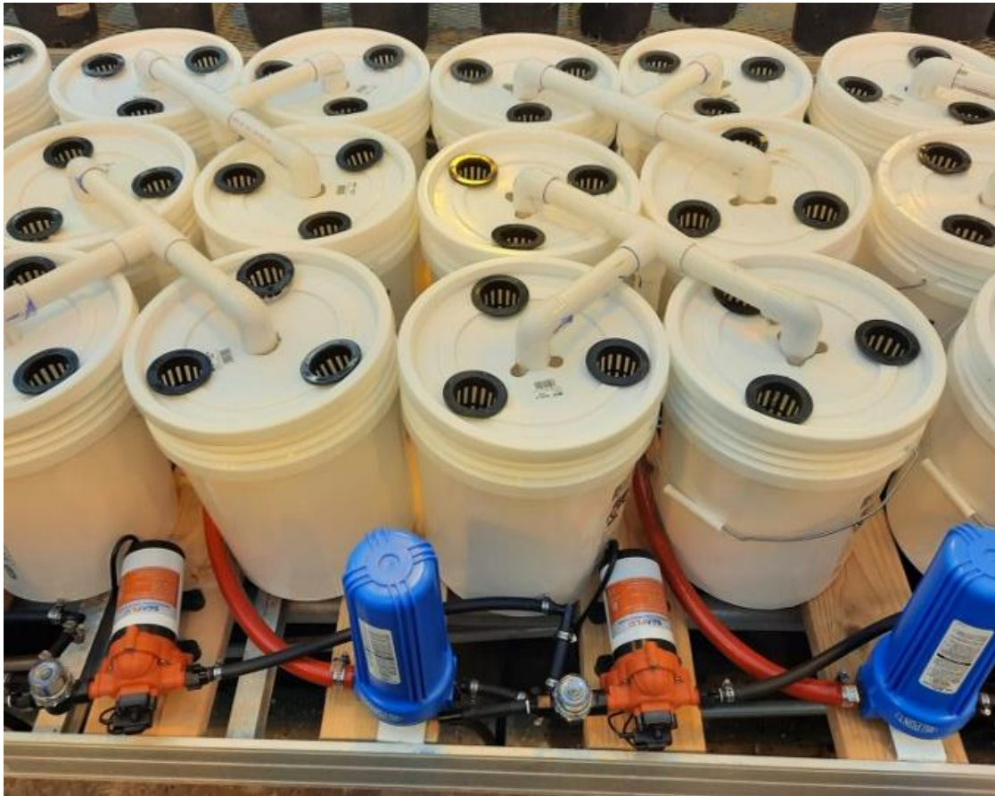
Figure 5. Complete aeroponic system. Plumbed from reservoir (beneath buckets), to pump (in orange), to filters (in blue) to buckets (through red hose and mated to PVC).
