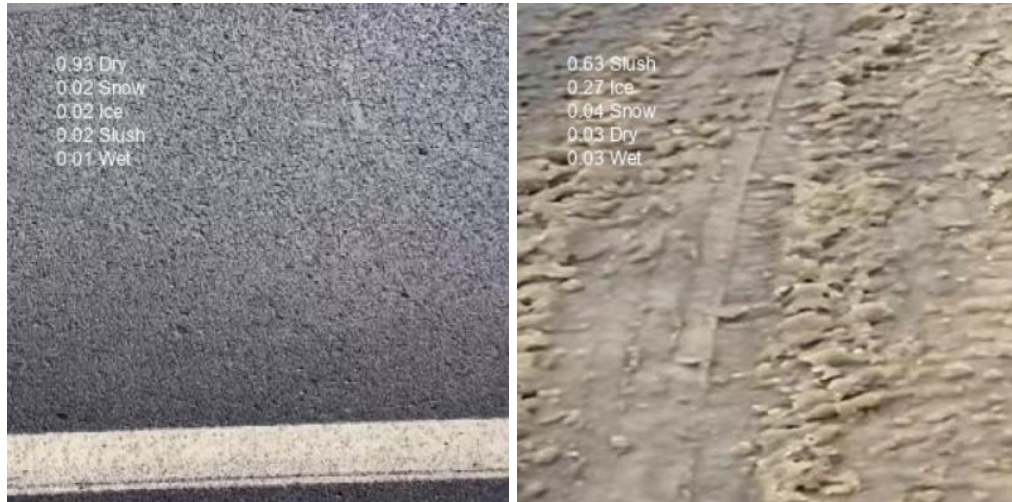
Figure 17. Examples of test images with the probabilities of all classes.
