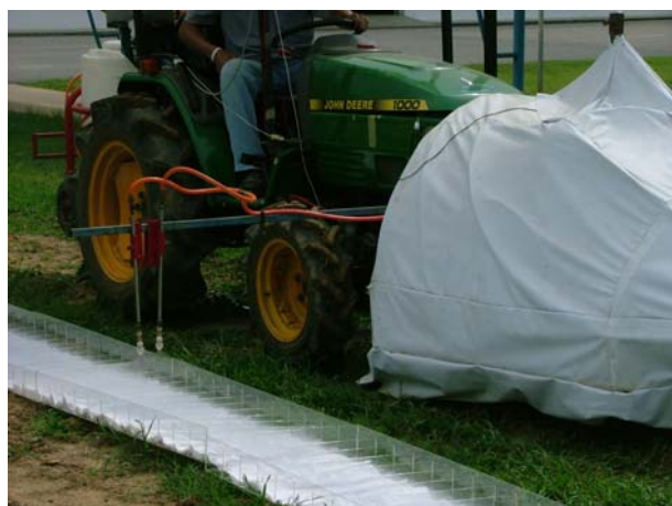
Figure 10. Test conducted for flow rate accuracy measurement with specially arranged corrugated plastic container with distance marks and nozzles on extended boom
