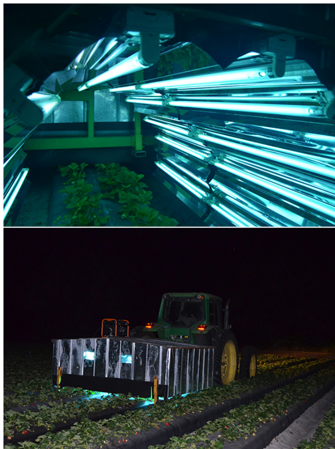
Figure 5. Tractor-drawn UVC array used in our first large-scale field trials on strawberries. Side-by-side arrays allowed two rows to be treated in each pass.
