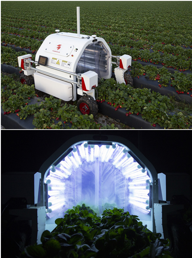
Figure 7. Thorvald, an autonomous robotic device developed in collaboration with SAGA Robotics in Norway, can carry and power the same UV array used in tractor drawn devices.
