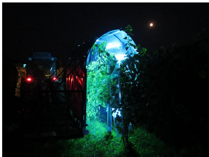
Figure 10. A tractor-drawn UVC lamp array used to treat grapevines at Cornell AgriTech. This same unit is also used to treat low-trellised hops.
