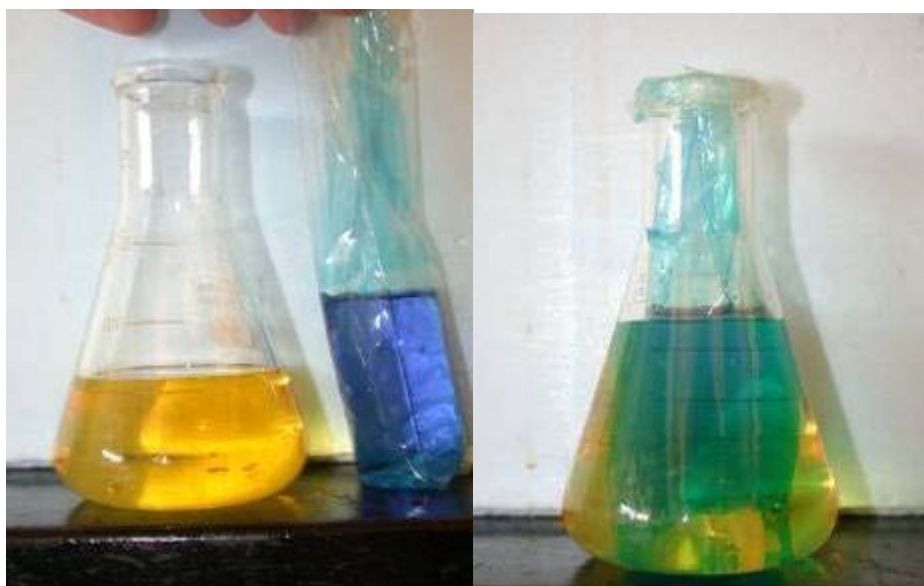
Figure 2 : Image of reactor vessel and dialysis tubing separate (left) and combined (right)
