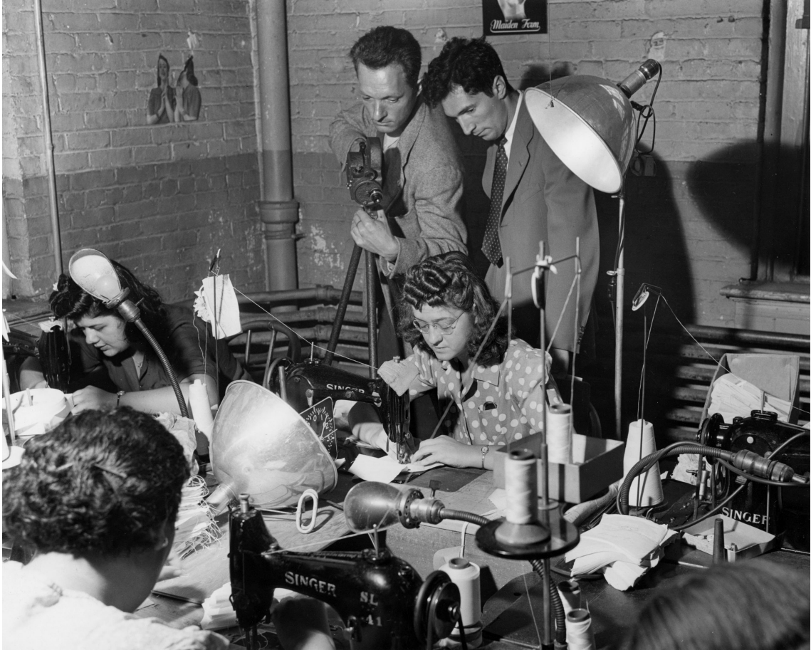
Figure 4.2: “Women sewing machine operators being filmed by two men for a time-motion study” 35mm negatives of photographs. Kheel Center for Labor-Management Documentation and Archives 5780 Box 84 Folder 5; Box 85 Folder 1
