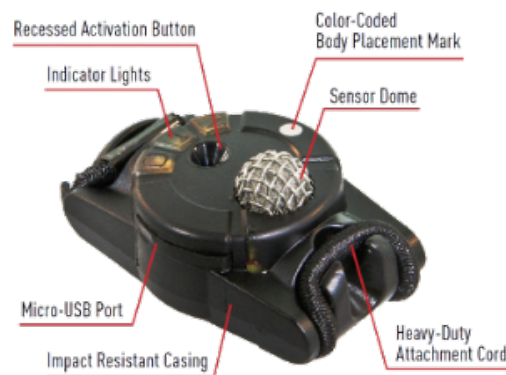
Figure 2.2: Blast Gauge sensor designed to monitor blast overpressure events in field environments, aiding in the assessment of TBI risk. Adapted from Blast Gauge System, by BlackBox Biometrics, n.d. ( https://blastgauge.com ). Copyright by BlackBox Biometrics. Used under fair use for educational purposes.
