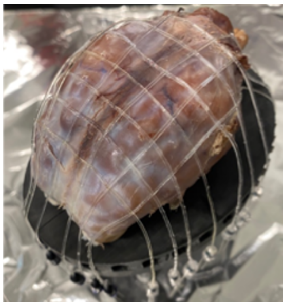
Figure 7.1: Overview image of preserved sheep brain setup and printed sensor holder.
