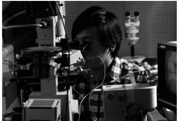
A researcher operates a micromanipulator used in embryo cloning and related research involving transfer of DNA among cells.
