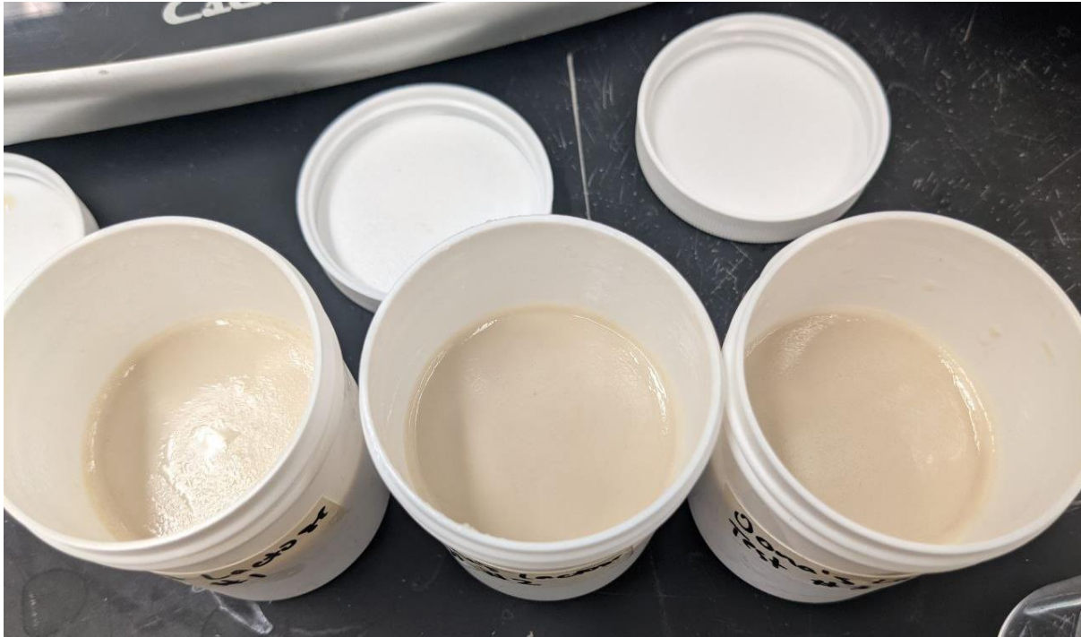
Figure 6. Visual Comparison of Plant-based Frozen Desserts Made With Oat Flour (Left), Rice Milk Flour (Middle), Commercial Dairy Ice Cream (Right).
