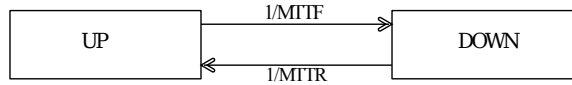
Figure 4.1: Markov Two State Generator Model. MTTF- mean time to failure and MTTR- mean time to repair
