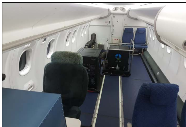
Figure 2.1.6. RANHD installed in Dash 8 aircraft
