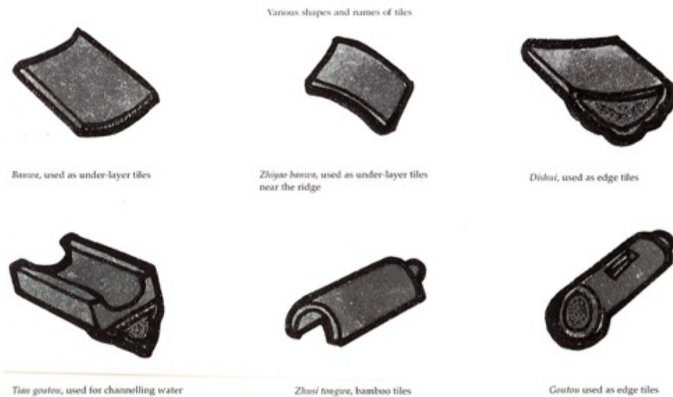
Figure 3.30. Glazed Ceramic Roofing Parts of the “Pan and Roll” Tiles (Source: Lip, E. (1995). Feng shui: environments of power: a study of Chinese architecture . London: Academy Editions, 14.)
