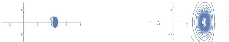
Figure 3.9: Left: c = -2.3 . The system quickly decays to the fixed point at \sqrt{-c} . Right: c = -2.6 . The system is spiraling outwards and accumulating on a limit cycle centered on \sqrt{-c} . A stability change has occurred very near the predicted value of c = -2.467 .
