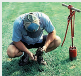
Sampling with the cup-cutter (bulb-planter) method. Photo: J. Grant, NYSIPM
