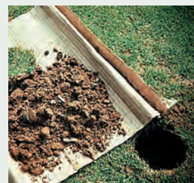
Sampling with the cup-cutter (bulb-planter) method. Photo: J. Grant, NYSIPM
