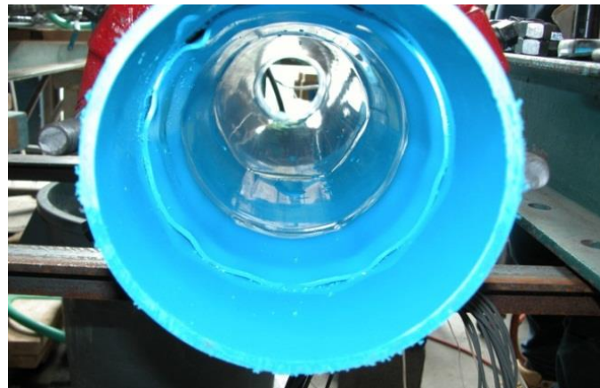
(b) Wrinkling of Specimen CT2 spigot
