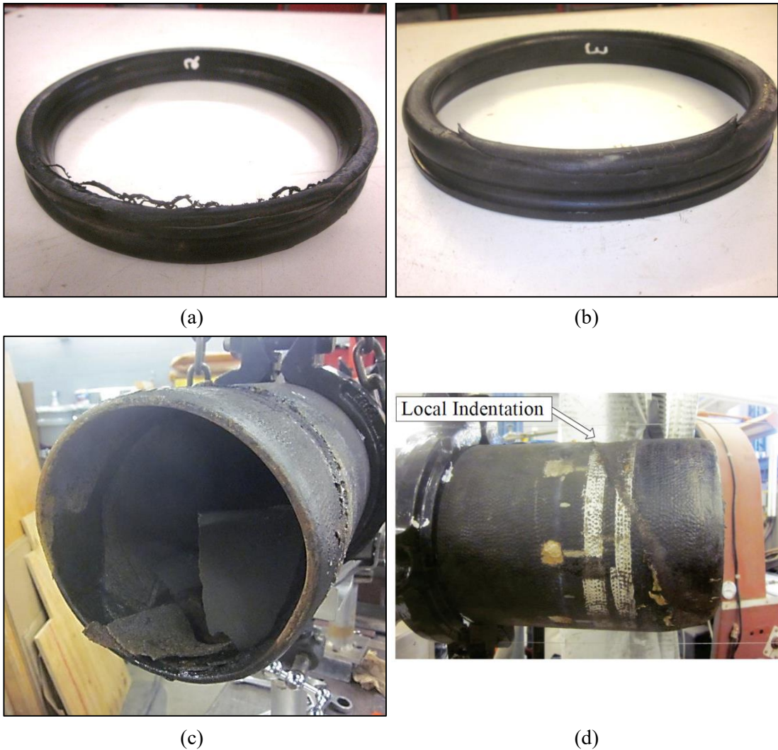
Figure 2.8. Gasket damage after: (a) 18-mm (0.7-in.); (b) 13-mm (0.5-in.) initial displacement tests; (c) deformed spigot after application of 26.7^\circ of rotation at axial displacement of 20.3 mm (0.8 in.); (d) Specimen B showing bending of spigot at both crown and invert
