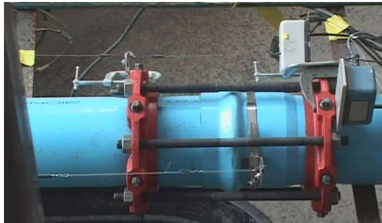
Figure 3.3. Specimen TT2 joint with restraint prior to tension test
