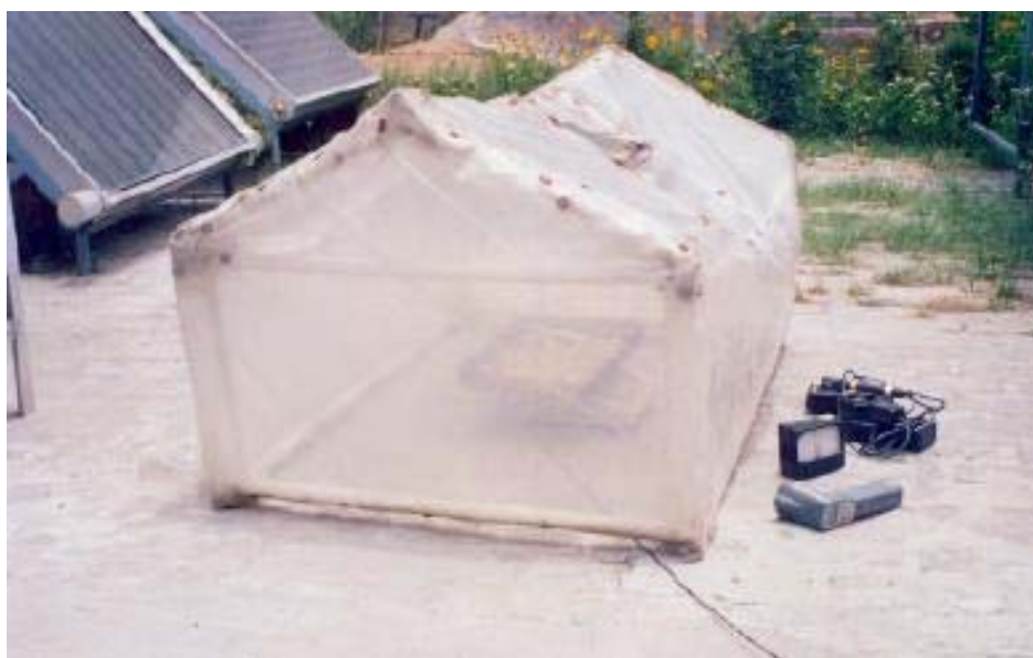
Figure 1. Experimental set-up for prawn drying inside greenhouse
