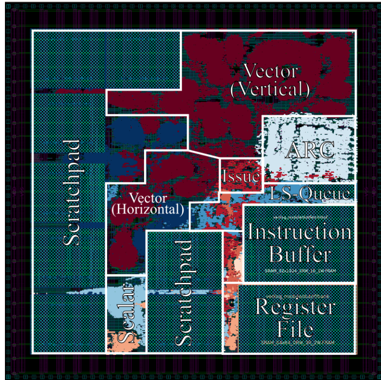
Figure 7.3: The generated layout of one VIP processing engine (PE).
