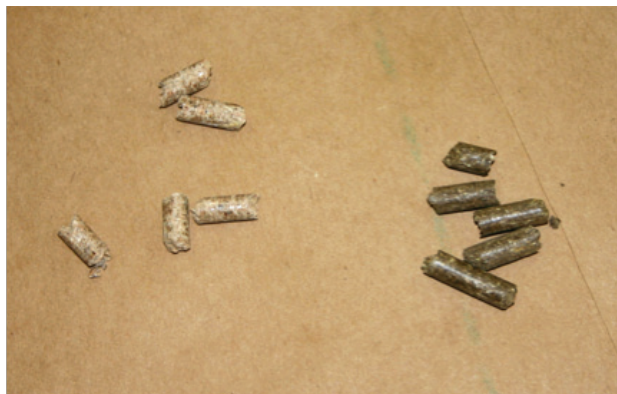
Wood pellets (L) and grass pellets (R). About ¼ - ½ inch in length
