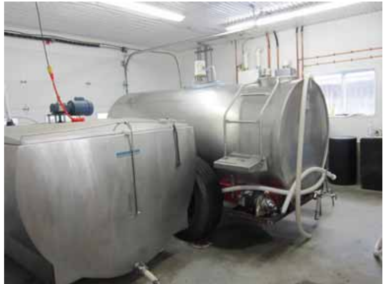
800 gal transport bulk tank – MR, waste, saleable milk mix is acidified.
