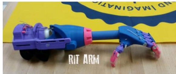
Figure 7: Example of an upper limb prosthetic for an individual who does not have a functional wrist or a palm. Source: enablingthefuture.org
