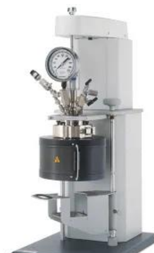
Figure 8 Hydrothermal Treatment Reactor Apparatus-Parr Reactor (Parr Instrument Company)
