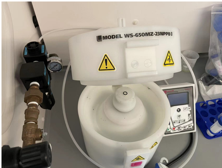
Figure 16: The Laurell WS-650-23 B spin coater
