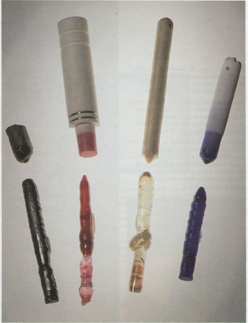
Figure 3. Some of the single crystals grown in the image furnace. The single crystals are shown below the corresponding feeding rods.
