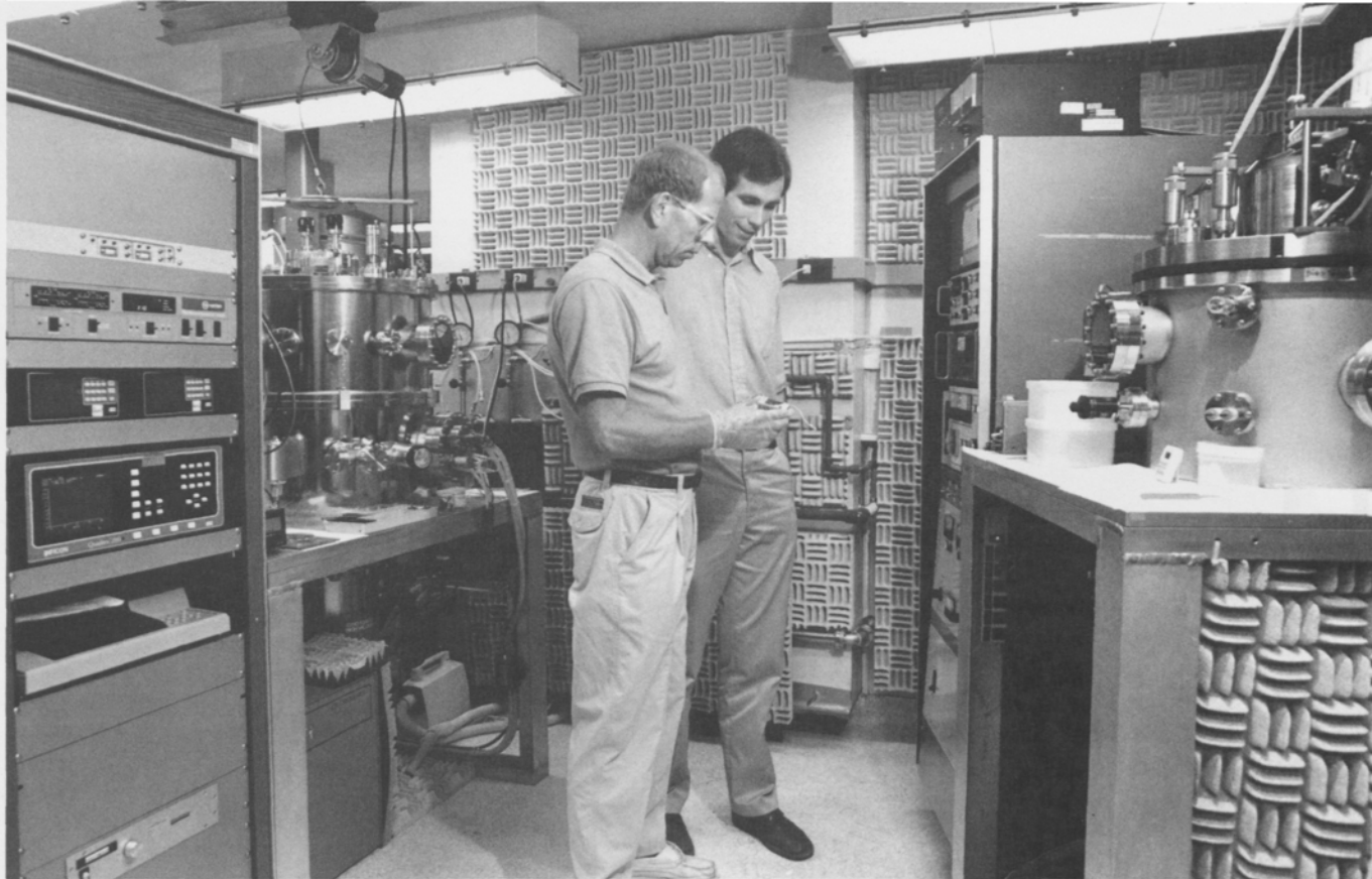
Gerhard Schmidt (at left) and graduate student David R. Peale are surrounded by equipment in the Technical Operations Laboratory. At left is a dual electron-beam deposition system; at right is a magnetron sputter system.
