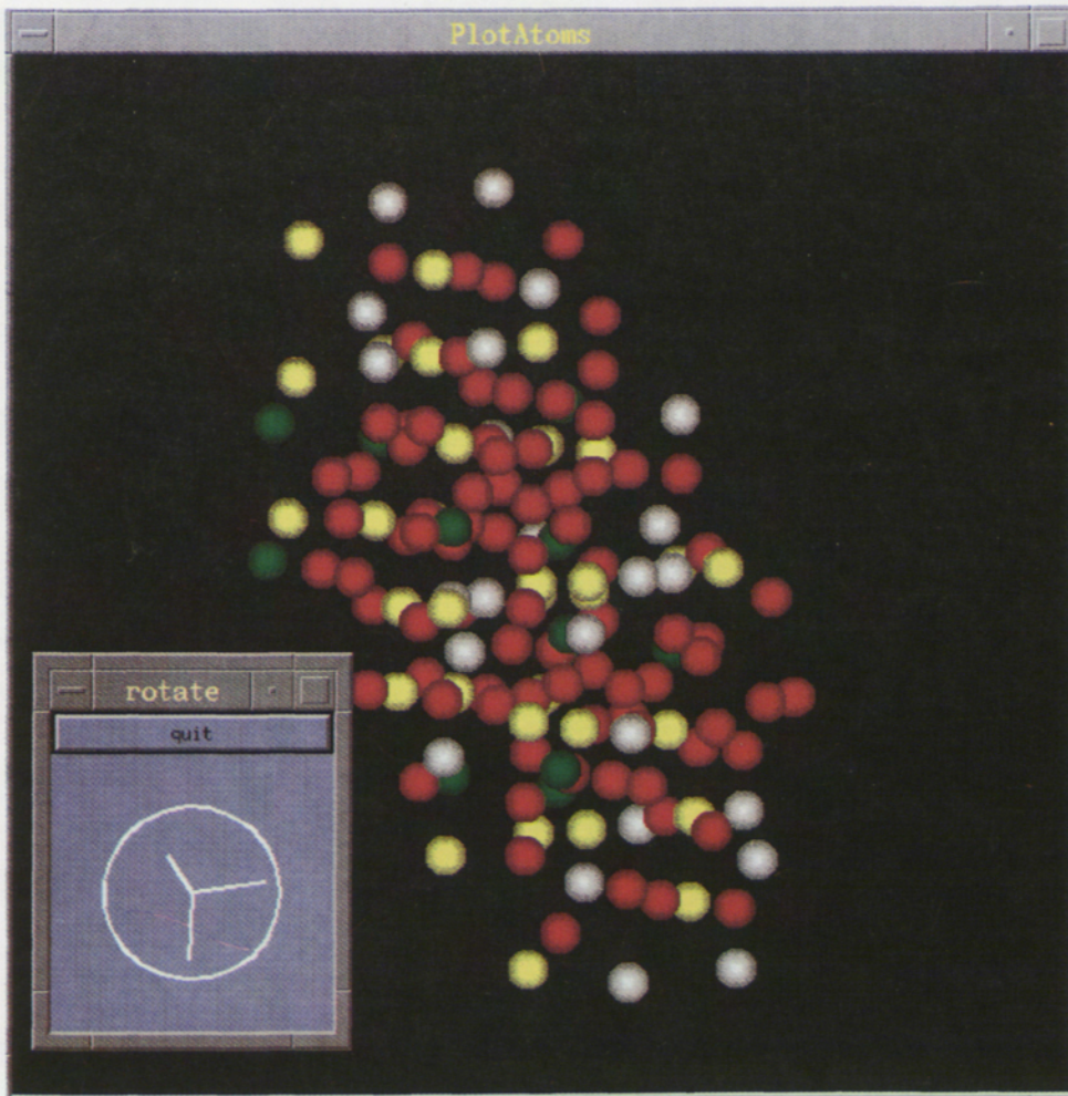
Figure 1. A unit cell from the crystalline phase of T_3 (AlMnZn), whose structure is believed to approximate that of decagonal quasicrystals such as Al_{65}Cu_{20}Co_{15} and AlCuNi.
