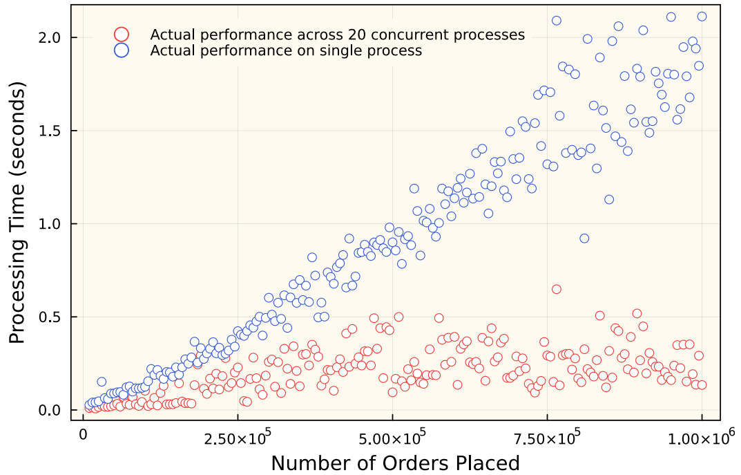
Figure 2.17: Comparison of actual processing time for order placement across 20 processes and single process
