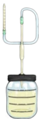
Figure 2. SO 2 tube apparatus. Reaction flask at bottom is connected to SO 2 detection tube via a condenser consisting of a volumetric pipette. (Image by Tammy Jones, Missouri Grape and Wine Institute)
