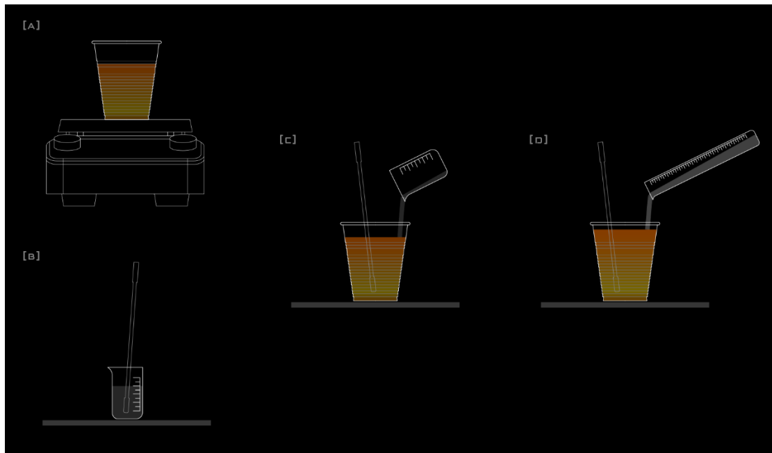
Figure 3-10: Final biomaterial composition used in the fabrication of the material studies. [a] powdered chitosan mixed with water, [b] hydrochloric acid mix, [c] acid added to dissolved chitosan solution, [d] regenerated silk solution added.
