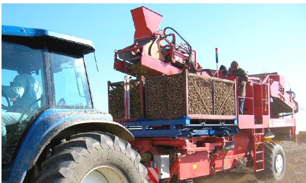
Figure 12. Harvesting machine with a device for filling two storage boxes with 1.5 t potatoes each
