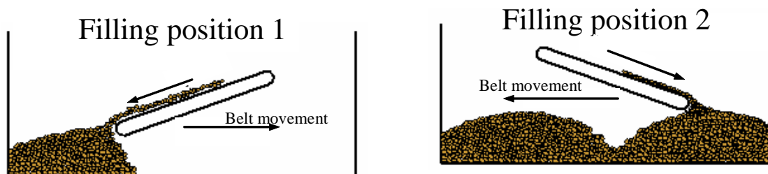
Figure 8. Formation of a low-additive area in the middle of the box in direct box filling attributable to the filling process
