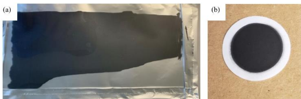
Figure 2.3: (a) Wet S/KB electrode slurry casted on Al foil. (b) Punched S/KB cathode disc for cell assembly
