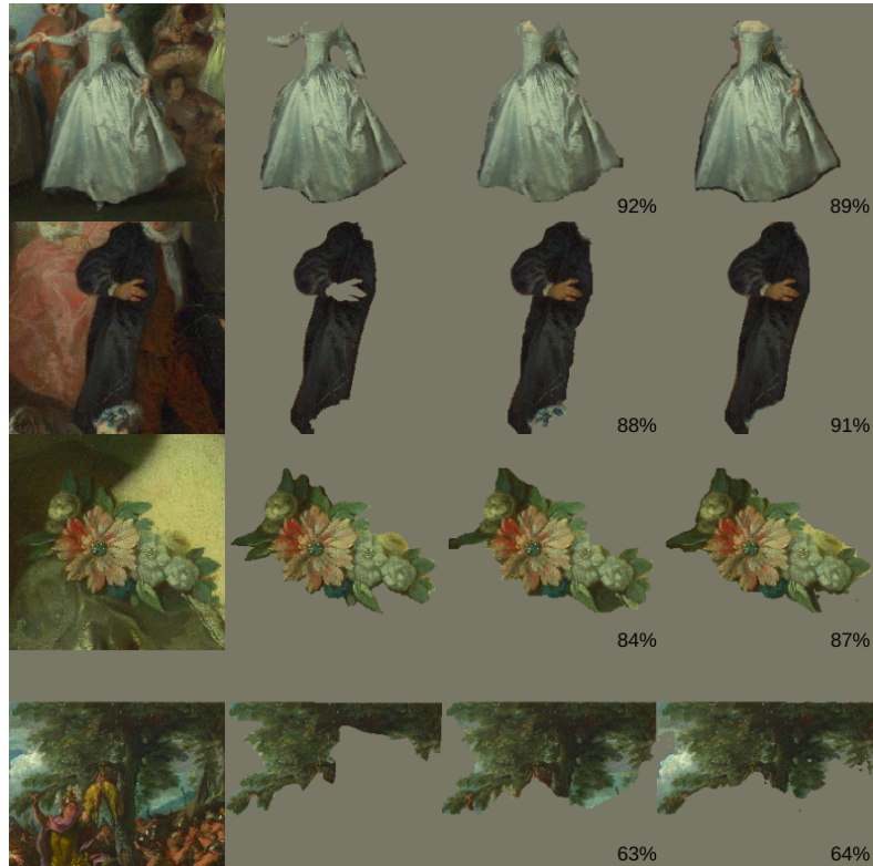
Figure 3.3: Extreme Click Segmentations. Left to right: Original Image, Ground Truth Segment, Grabcut Extr Segment, DEXTR COCO Segment. Both Grabcut and DEXTR use extreme points as input. For evaluation, the extreme points are generated synthetically from the ground truth segments. In practice, extreme clicks can be crowdsourced. Bottom-right corner shows the IOU for each segmentation.
