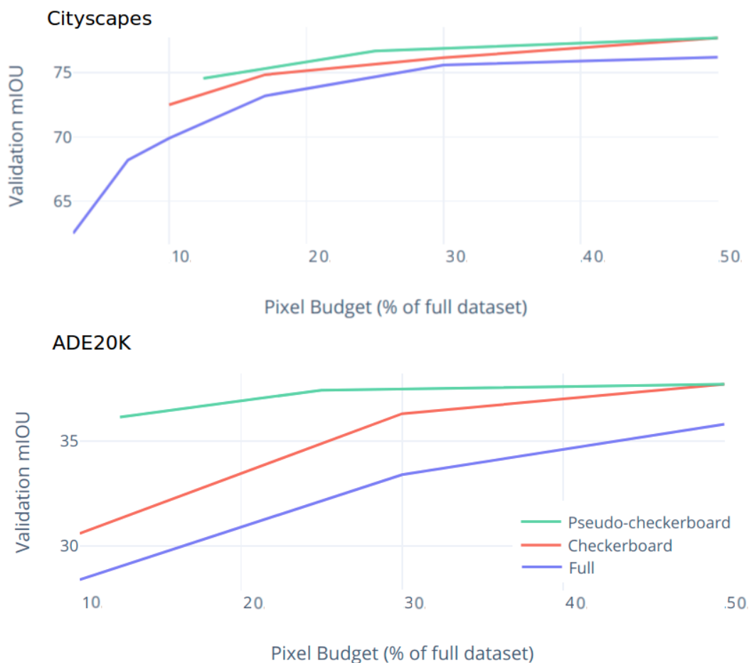
Figure 2.7: Semantic segmentation performance. Training images are annotated with different pixel budgets. Pseudo-checkerboard block annotation outperforms checkerboard and full annotation.
