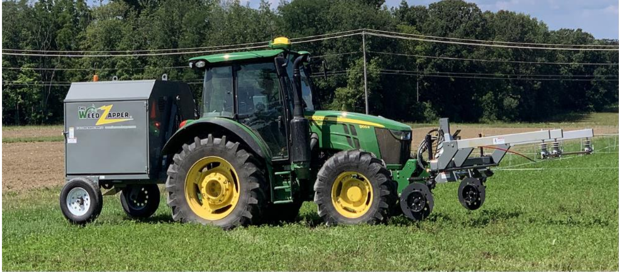
Figure 2: The model 6R30 Weed Zapper used in this experiment. The generator is attached to the back of a John Deere 5100R tractor with a 3-point hitch. The 4.6 m electric copper boom is attached to the front of the tractor with a 3-point hitch. The Weed Zapper was purchased from Old School Manufacturing, LLC in Sedalia, MO.
