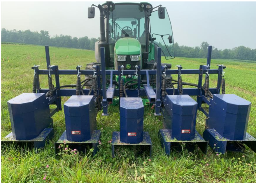
Figure 1: The inter-row mower used in this experiment, attached to a John Deere 5100R tractor with a 3-point hitch. The mower is powered with a hydraulic system and was custom made by IRM X4, R-Tech Industries Ltd. in Homewood, MB.
