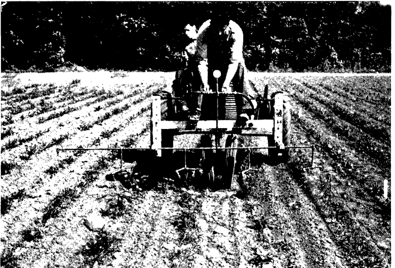
FIG. 11.—Applying salt spray to weed beets. Rigid copper tube boom with two nozzles per row makes a simple type of construction. Operator is controlling valves that determine flow of solution to boom for spraying this experimental plot.
