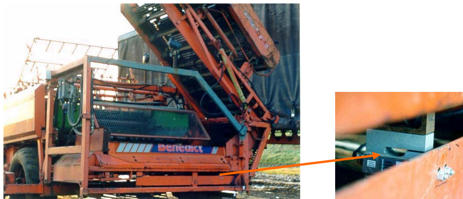
Fig. 5. Diagram of the load cell supporting system in the potato harvester
